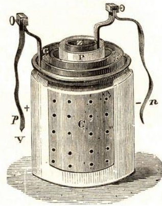
Figure 2 : The Daniell cell, a wet storage battery.
